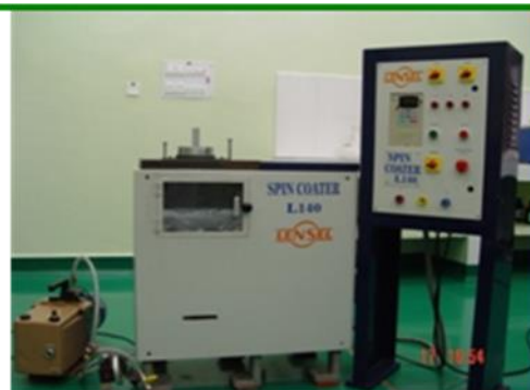
Sol-gel spin coater (at RRCAT) holding a laser rod for AR coating
