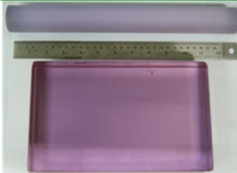
Optically polished Nd:glass slab & machined glass rod (at RRCAT)
