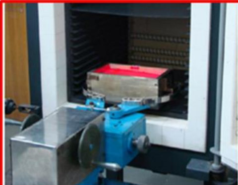
Transfer of cast glass to annealing furnace (at CGCRI)
